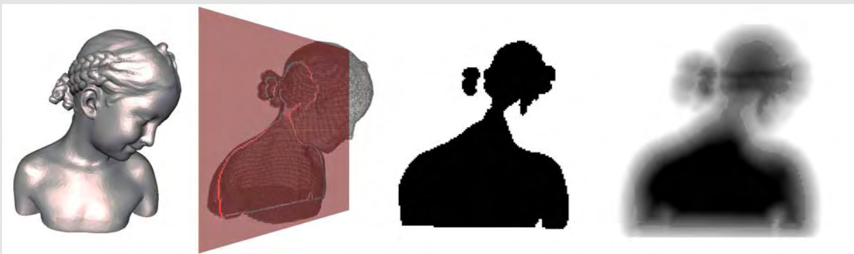
Rasterization of the "bimba" model over a cut plane and blurred shape
