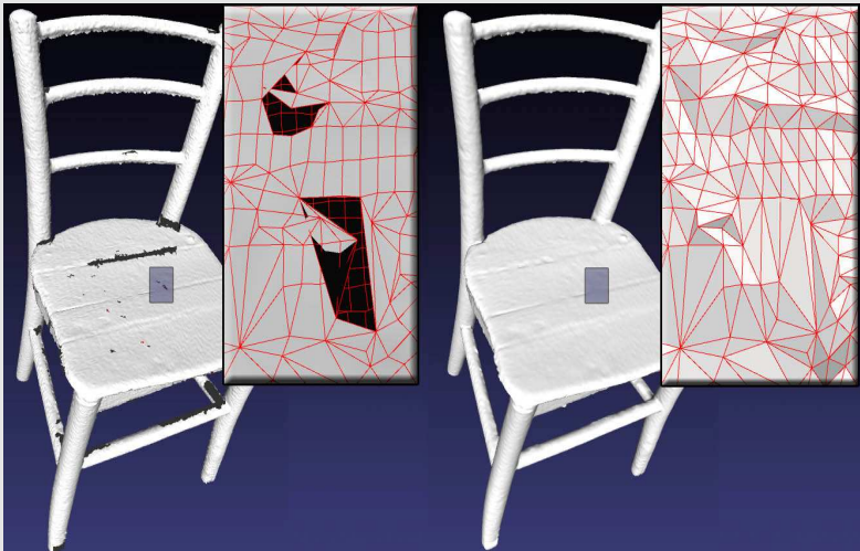
The model of a chair repaired through our new algorithm
